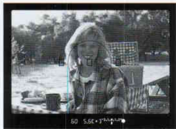
Partial metering circle
